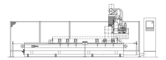
Weeke's Venture 1 is a flexible CNC machining center designed primarily for routing, boring, and grooving of flat panel components without special workpiece fixtures.
