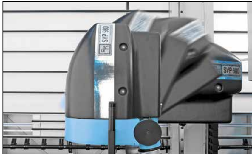
Motorized Saw Head rotation from Control Panel
