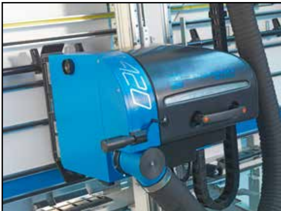
Ergonomic Saw Head with energy chain to safely house all cables
