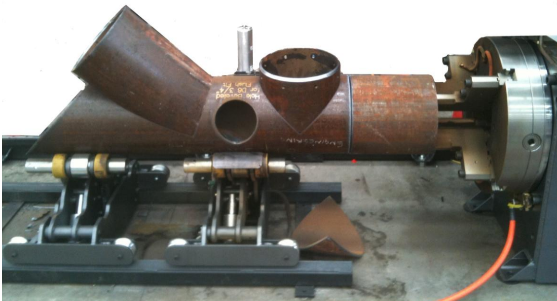
Picture showing assortment of cut parts, put together after cutting of pipe, plasma machine not shown
