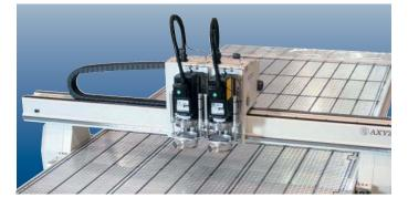
Choose a single, double or even triple-head carriage for multiple tasking operations, popular for applications that typically require only two or three tooling processes. Multi-head machines can be faster and more economical than one with an automatic toolchange system. HSD router spindles feature a simple and powerful quick-release tool change system. The manual tool-change Elte spindles provide a conventional collet and covernut alternative.
