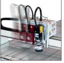
Multiple gantries on a single machine bed offer the user flexibility in machine use. Run different operations at either end of the machine, or park one gantry for large job processing over virtually the entire machine length.
